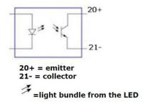
The pulse output is 1000 per kWh and is settable using the MBus communication protocol. The table below outlines the possibilities.
