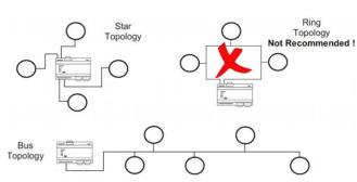
The cable resistance, therefore, limits the maximum possible cable length from the MBus Master / Repeater to the device with the largest distance away from it (largest cable segment). The cable segment length is the distance from the MBus Master to the MBus device furthest away.
